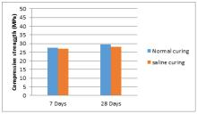
Fig.4. Compressive strength for Mix 2
