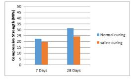
Fig.5. Compressive strength for Mix 3
