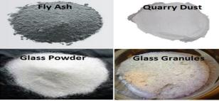
Fig.1. Photographs of Fly ash, Quarry dust, glass powder and glass granules
